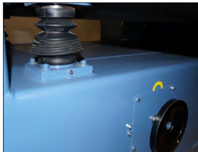
Hand Wheel: Adjusting the sanding tolerance easily.
