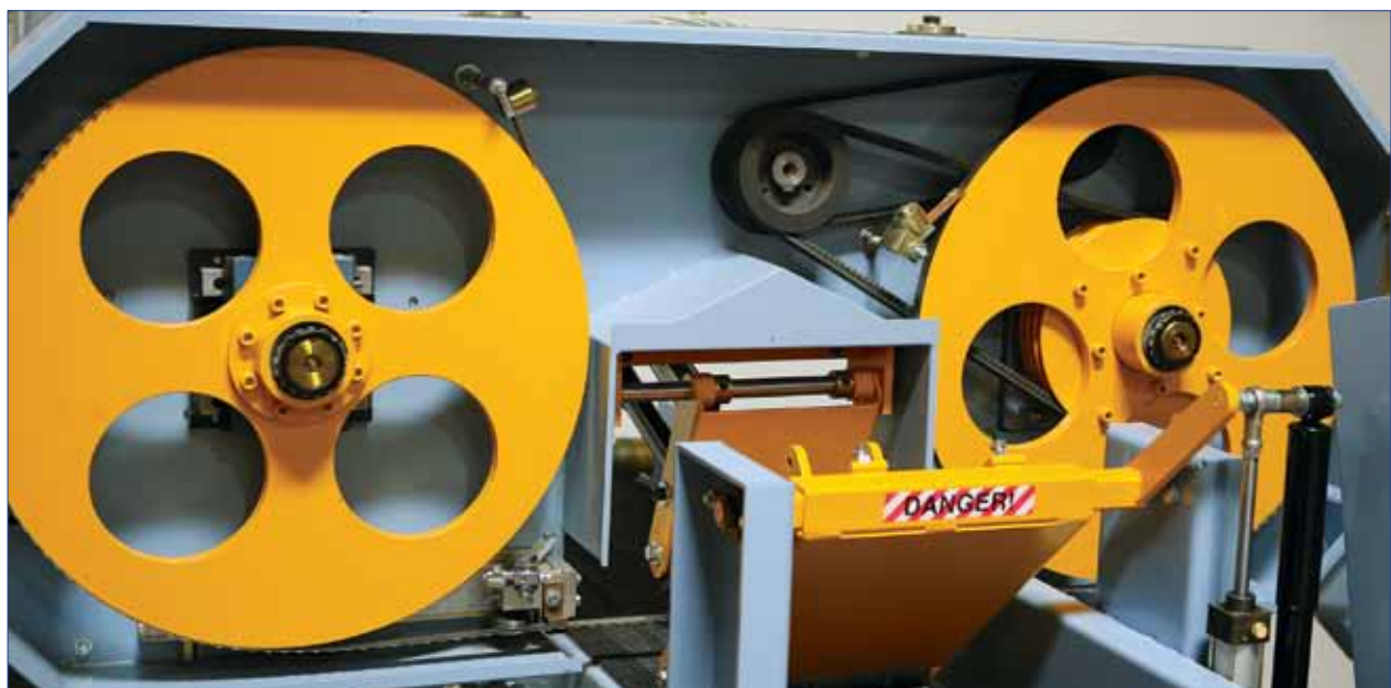
Linear bearing guides support the massive band wheels to ensure longevity and negate saw vibration.
