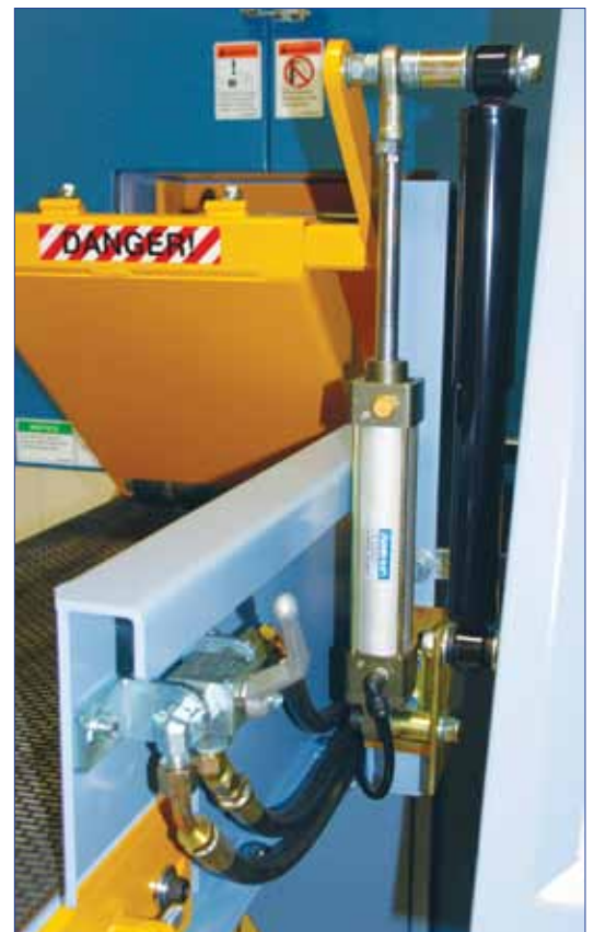
Front hold down pressure is adjustable by an air cylinder acting with a shock absorber to securely hold the material to the conveyor ensuring a superior cut.
