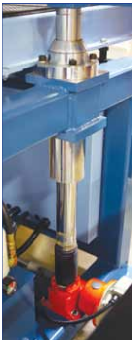
Massive 2-3/8" chrome steeled lift rods are guided through a 15" long housing to ensure rigid support of the band mill.
