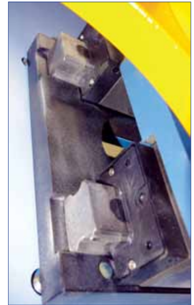
Linear bearing guides support the massive band wheels to ensure longevity and negate saw vibration.
