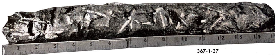
Steel Shafting, 1 15/16" diameter x 15" long, that was accidentally fed to a Wood Hog and ended in the Metal Catcher. No damage was done to the machine.
