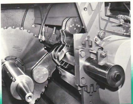
Top arbor stationary saw guides, infeed only, are available to provide net cuts from %" minimum to as wide as required.
