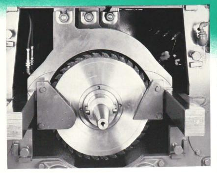
Top arbor saw shifter guide arms mounted in edger in sawing position. Each shifter is bolted to a clamp assembly which is mounted on a chromed, top-mounted saw shifter shaft, and is supported front and rear on chromed, guide support bars.
