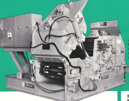
A model 3 TA 36 (SB) top arbor edger with slat bed feed system, splined arbor, 4 shifting saws, tip-up babbitt-type shifters, side mounted setworks for saws, and a clamshell opening for easy access to saws and guide units.
